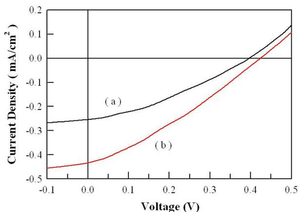
Fig. 5 *J-V* characteristic curves of two Si QDSSCs.
