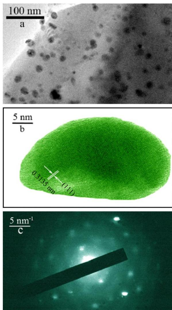
**Fig. 3** TEM images of Si quantum dots prepared from the porous Si film: (a) low resolution, (b) high resolution, (c) selected area electron diffraction pattern.
