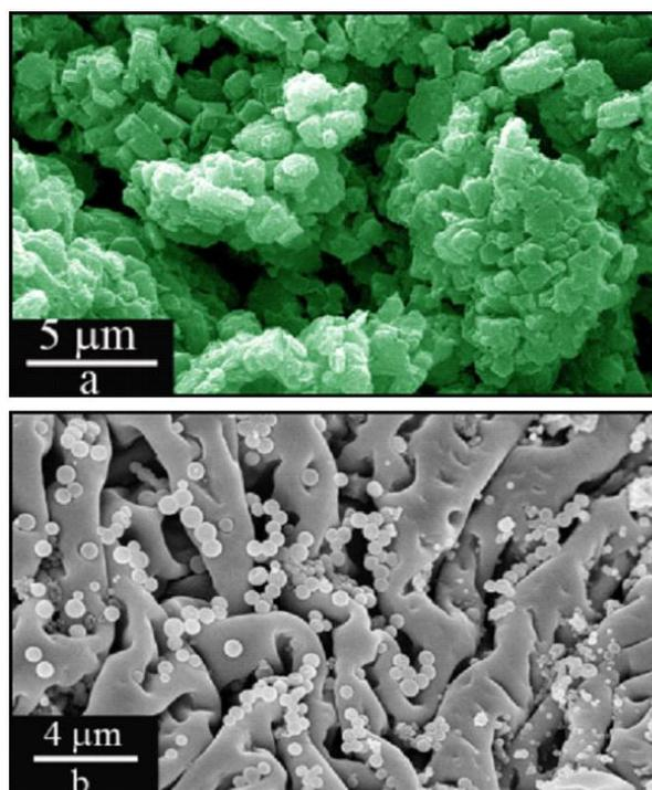
**Fig. 2** SEM micrographs of TiO<sub>2</sub> porous film before (a) and after (b) the Si quantum dots sensitization.
