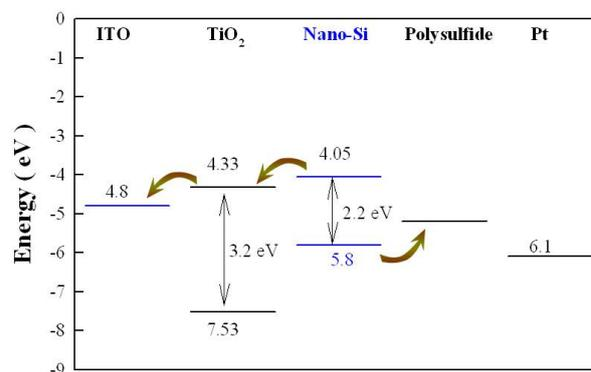
Fig. 7 Schematic illustration of the energy diagram of Si QDSSC.
