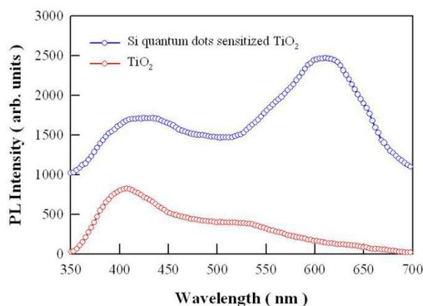
**Fig. 4** PL spectra of TiO<sub>2</sub> porous film (a) and Si quantum dots sensitized TiO<sub>2</sub> film (b).
