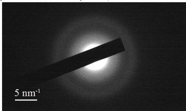
Fig. 8 Selected area electron diffraction of Si quantum dots.
