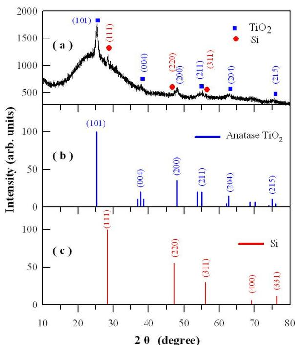
**Fig. 1** XRD spectra of Si quantum dots sensitized TiO<sub>2</sub> thin film (a), anatase titania (PDF#21-1272) (b) and crystalline Si (PDF#27-1402) (c).
