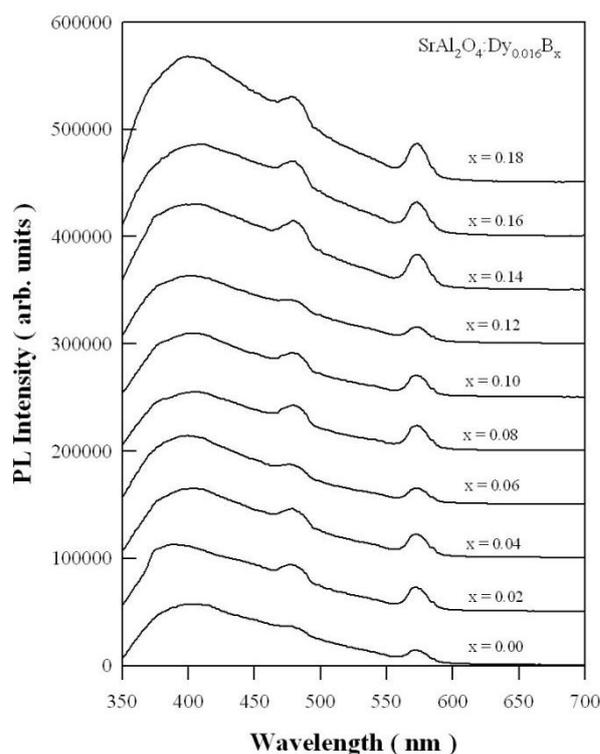
Fig. 3 Evolution of the PL spectra of DSAO with the concentrations of  $\text{H}_3\text{BO}_3$  in the starting materials.
