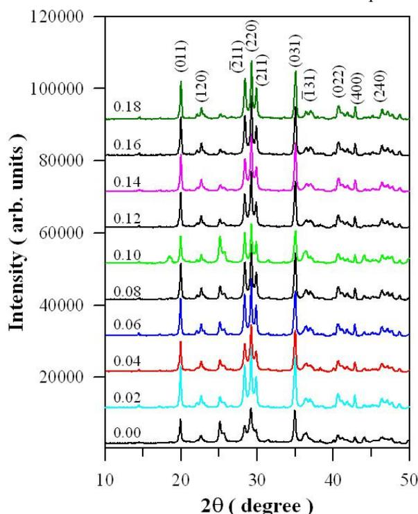
Fig. 1 XRD curves of the DSAO: $\text{B}_x$  ( $x = 0.00$ – $0.18$ ) prepared with different  $\text{H}_3\text{BO}_3$  concentrations in the starting materials.
