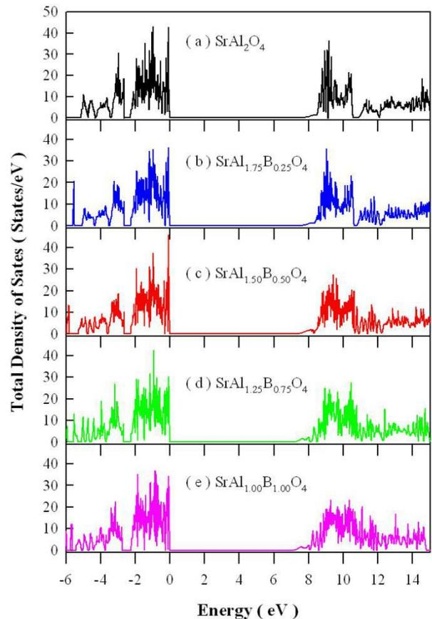
**Fig. 5** Calculated densities of states of SrAl<sub>2</sub>O<sub>4</sub> (a), SrAl<sub>1.75</sub>B<sub>0.25</sub>O<sub>4</sub> (b), SrAl<sub>1.50</sub>B<sub>0.50</sub>O<sub>4</sub> (c), SrAl<sub>1.25</sub>B<sub>0.75</sub>O<sub>4</sub> (d), SrAl<sub>1.00</sub>B<sub>1.00</sub>O<sub>4</sub> (e).
