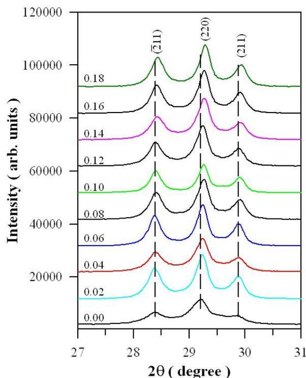
Fig. 2 Evolution of zoomed XRD curves of the DSAO with the concentration of  $\text{H}_3\text{BO}_3$  in the starting materials.
