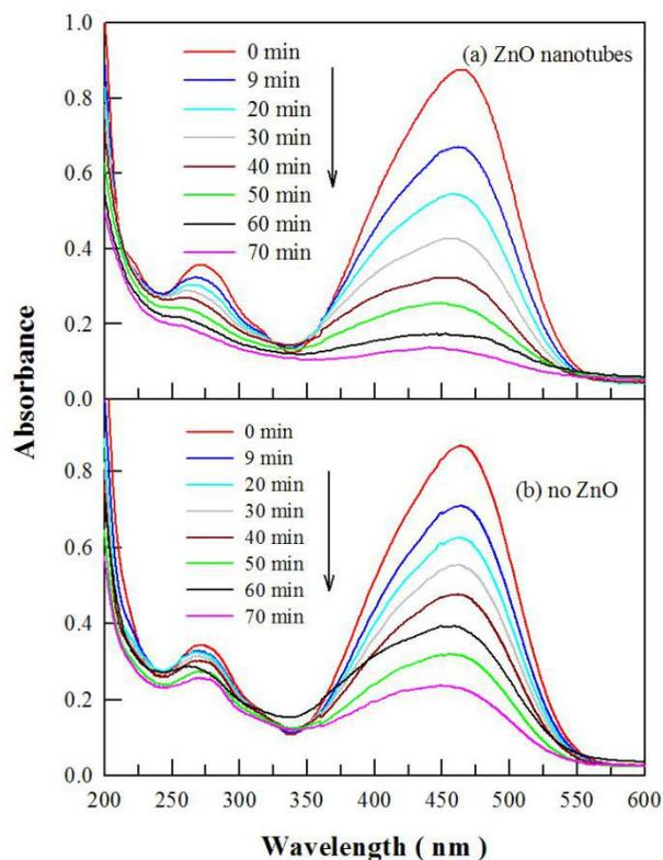
Fig. 5 Evolution of the absorption spectrum of methyl orange solution with the irradiation time of the high-pressure mercury lamp: (a) in the presence of vertically aligned ZnO nanotubes; (b) in the absence of the ZnO nanotubes.
