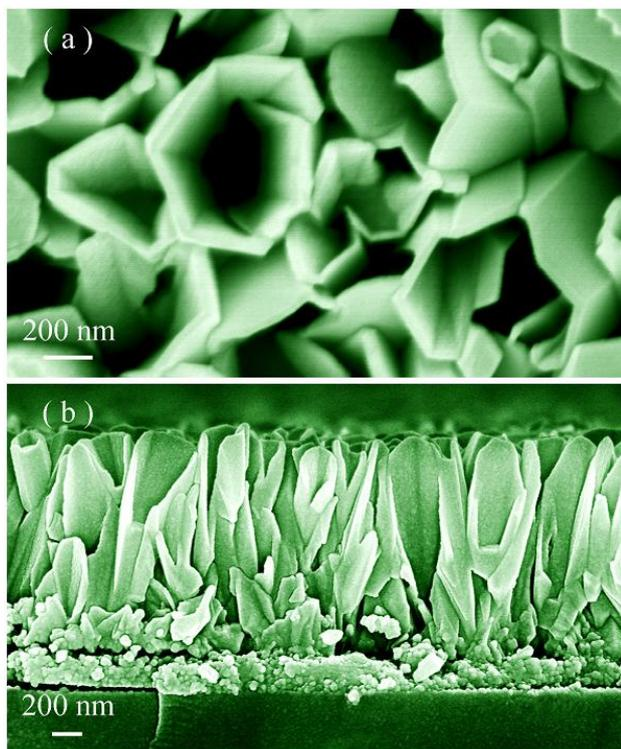
**Fig. 2** Top-view (top panel) and cross-sectional (bottom panel) SEM micrographs of the vertically aligned ZnO nanotubes grown on a glass substrate.
