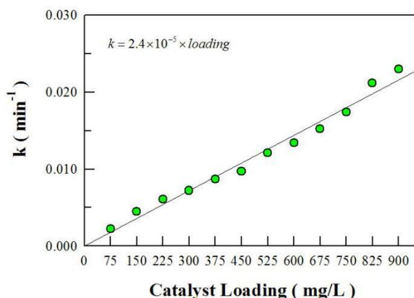
Fig. 7 Catalyst loading dependent photocatalytic rate constant of the vertically aligned ZnO nanotubes.
