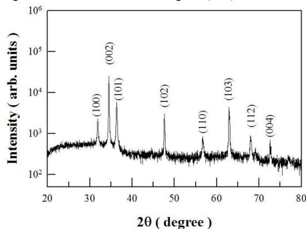
**Fig. 3** XRD spectrum of vertically aligned ZnO nanotubes grown on a glass substrate.
