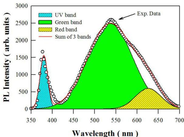
Fig. 4 PL spectrum of vertically aligned ZnO nanotubes and its three Gaussian components.
