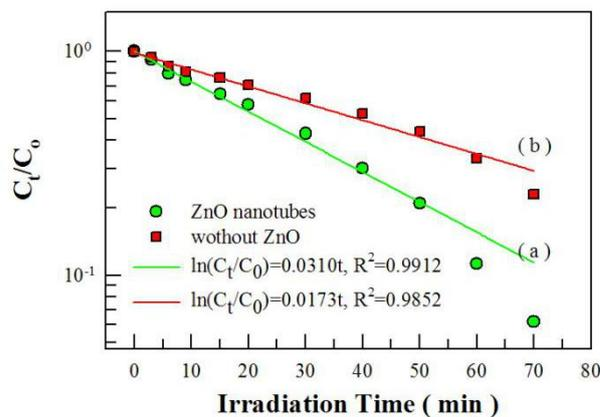
Fig. 6 Semi-log plots of  $C_t/C_0$  as a function of irradiation time of the high-pressure mercury lamp: (a) in the presence of ZnO nanotubes (circles); (b) in the absence of ZnO nanotubes (squares).
