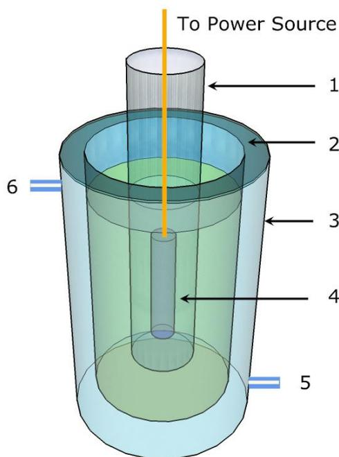
**Fig. 1** Schematic illustration of the photocatalytic reactor. 1: an inner cylindrical quartz tube ( $\phi 55$  mm) to house the high-pressure mercury lamp. 2: a middle cylindrical glass tube ( $\phi 85$  mm) to reserve the dye solution. 3: an outer cylindrical glass tube to contain the cooling water. 4: a high – pressure mercury lamp. 5: inlet of the cooling water. 6: outlet of the cooling water.
