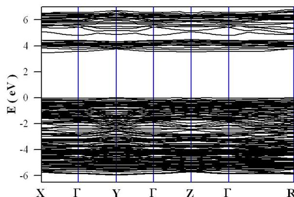
**Fig. 6** Calculated band structures and density of states of defect-free triclinic ZnMoO<sub>4</sub>.
