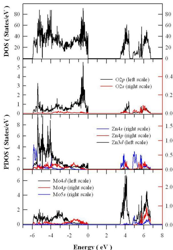
**Fig. 7** Top panel: calculated total density of states of defect-free triclinic ZnMoO<sub>4</sub>. The rest three panels: calculated partial density of states of defect-free triclinic ZnMoO<sub>4</sub>.
