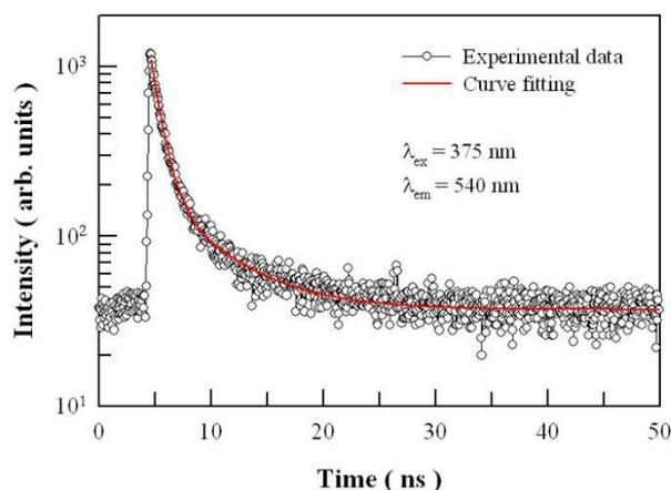
**Fig. 5** Time-resolved PL spectra of ZnMoO<sub>4</sub> grown by sintering the precipitate at 500°C for 2 h.
