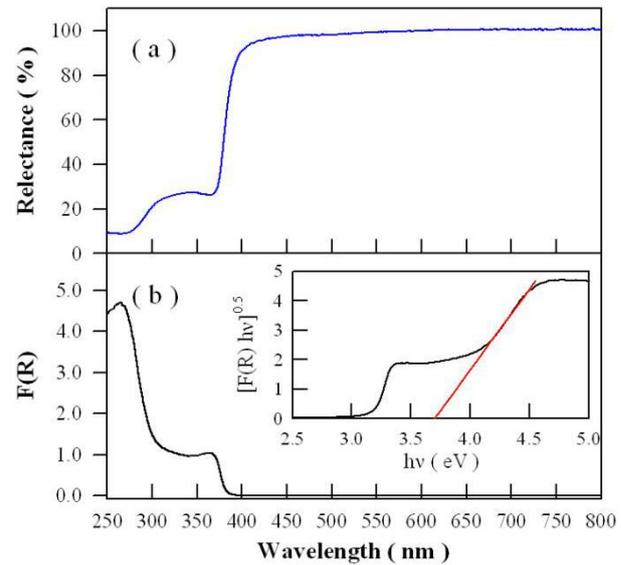
Fig. 3 Reflectance spectrum (a) and absorption spectrum (b) of ZnMoO<sub>4</sub> microcrystal grown at 500°C for 2 h.
