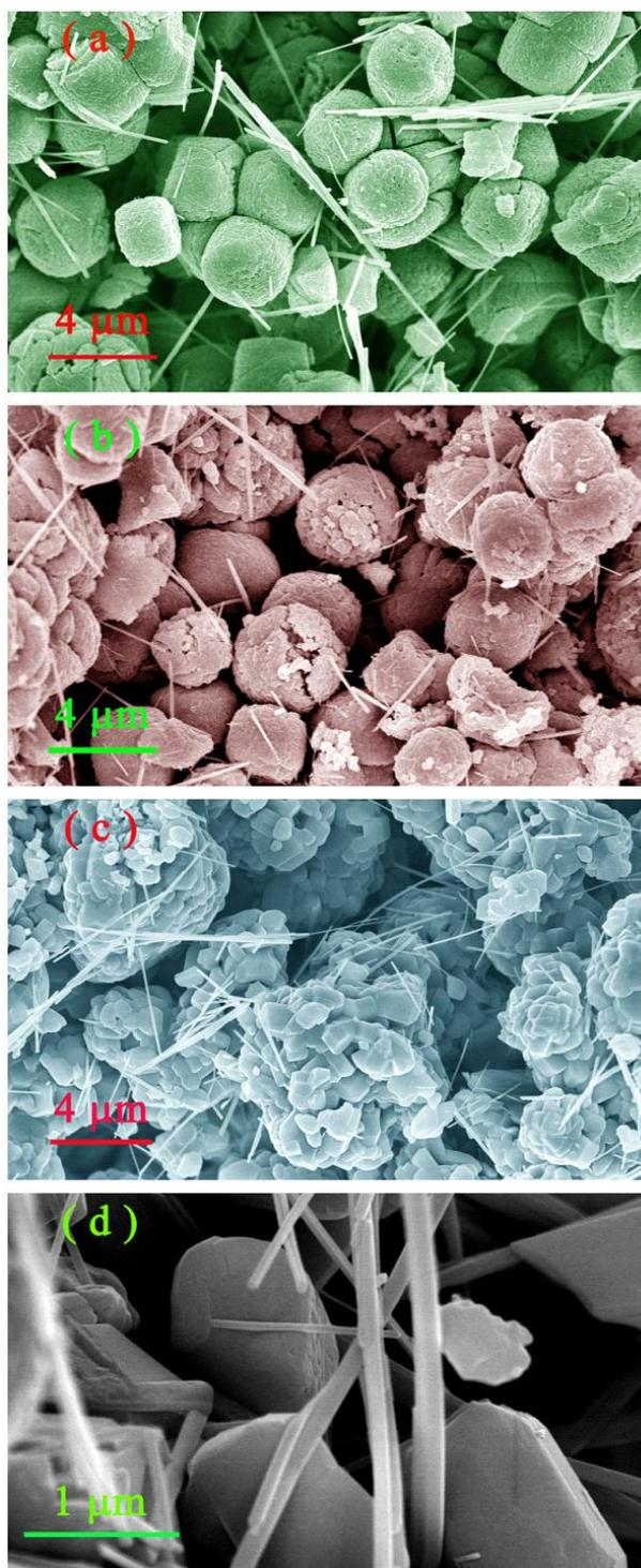
**Fig. 1** SEM micrographs of  $\text{ZnMoO}_4$  grown by sintering the precipitate at different temperatures for 2 h: (a) 300°C; (b) 400°C; (c) 500°C; and (d) 600°C.
