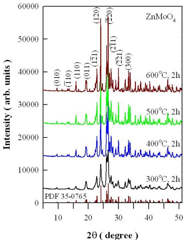
Fig. 2 XRD curves of the triclinic ZnMoO<sub>4</sub> grown by sintering the precipitate at 300, 400, 500 and 600°C for 2 h.
