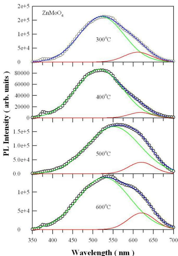
**Fig. 4** PL spectra of ZnMoO<sub>4</sub> microcrystals grown by sintering the precipitate at 300, 400, 500 and 600°C for 2 h. The excitation wavelength was 325 nm.
