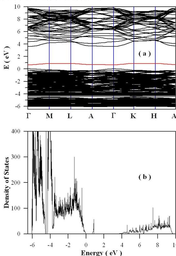
Fig. 4 DFT calculated bandstructures and density of states of Zn-rich and oxygen-deficient ZnO<sub>0.98</sub>.
