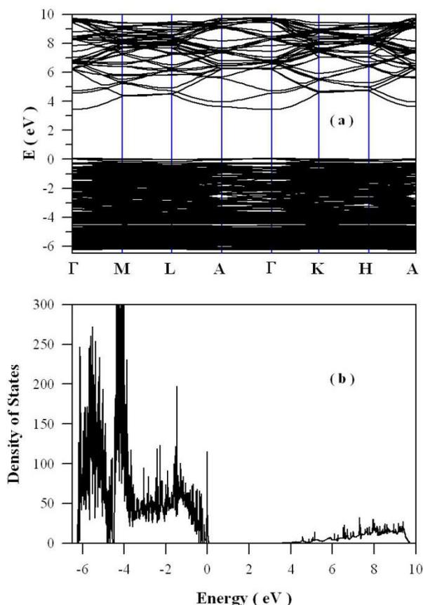
**Fig. 5** The DFT calculated bandstructures and density of states of O-rich and Zn-deficient  $\text{Zn}_{0.98}\text{O}$ .
