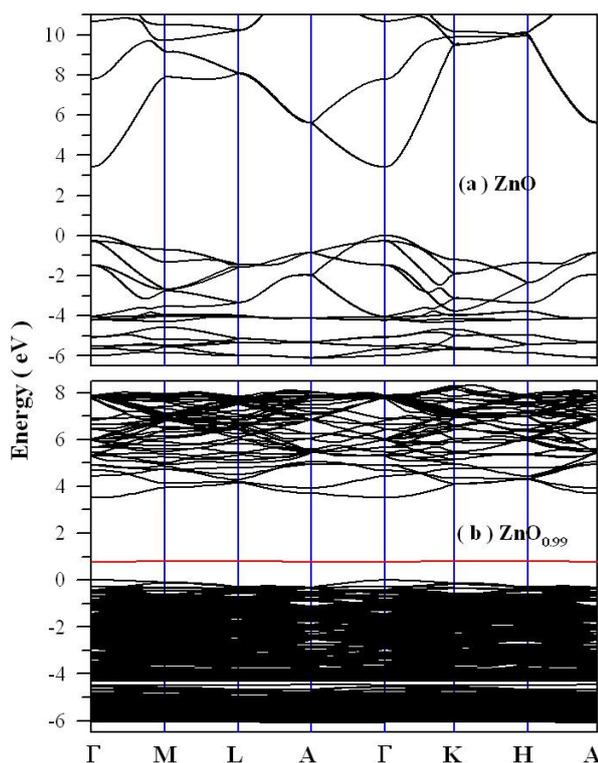
Fig. 3 DFT calculated bandstructures of perfect ZnO (upper panel) and oxygen-deficient ZnO<sub>0.99</sub> (lower panel).
