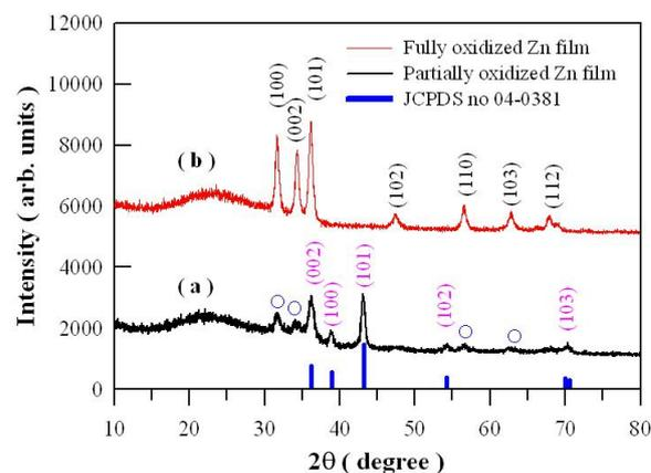
Fig. 1 XRD spectra of Zn-rich ZnO film (a) and O-rich ZnO
